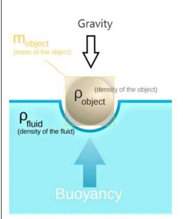
• The principle behind buoyancy is described by **Archimedes' Principle**, which states that an object submerged in a fluid experiences an upward force equal to the weight of the fluid displaced by the object. If the upward buoyant force is greater than the object's weight, the object will float; if the weight is greater, the object will sink.
